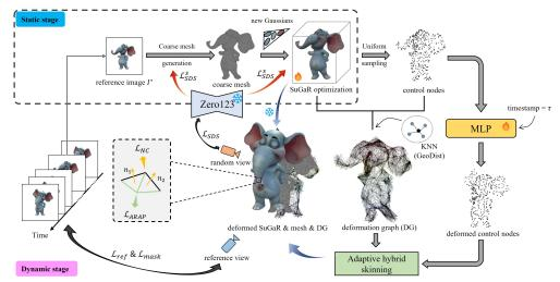
Figure 2: **Overview of DreamMesh4D.** In static stage shown in top left part, a reference image is picked from the input video from with we generate a Gaussian-mesh hybrid representation through a image-to-3D pipeline. As for dynamic stage, we build a deformation graph between mesh vertices and sparse control nodes, and then the mesh and surface Gaussians are deformed by fusing the deformation of control nodes predicted by a MLP through a novel adaptive hybrid skinning algorithm.
